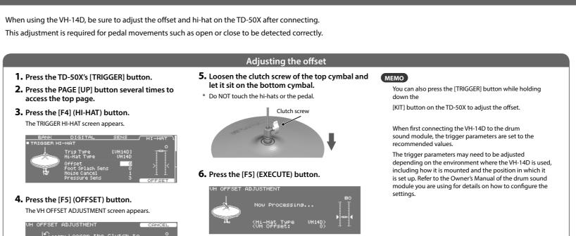
The "VH offset" parameter is set automatically (approx. 3 When the adjustment is complete, the [TRIGGER] button
