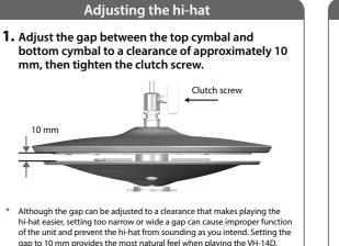
hi-hat easier, setting too narrow or wide a gap can cause improper functi gap to 10 mm provides the most natural feel when playing the VH-14D. 2. Change the spring tension by adjusting the hi-hat
