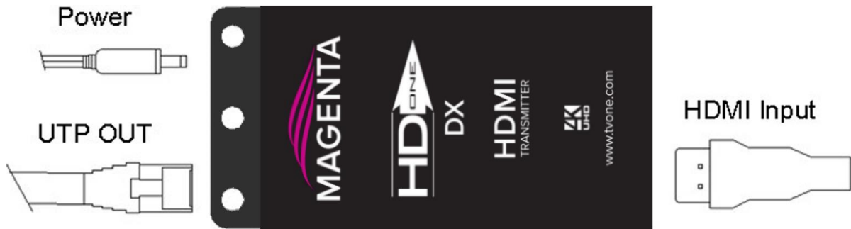
Figure 1 - Connections on the Transmitter
